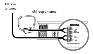
The supplied antennas provide a simple way to listen to AM and FM radio. If you find that reception quality is poor, an outdoor antenna should give you better sound quality—see *Connecting external antennas* on page 12 for more on how to do this.
